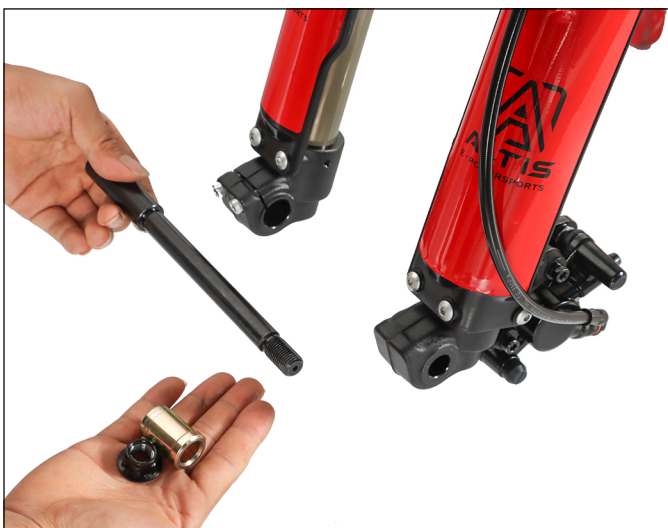
15. Disassemble the tire mounting rod to install screws
