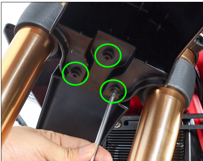
9. Fix the mudguard screws
