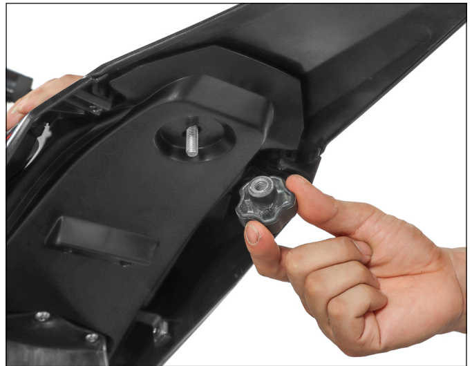
24. Open the screw cap at the bottom of the rear tail
