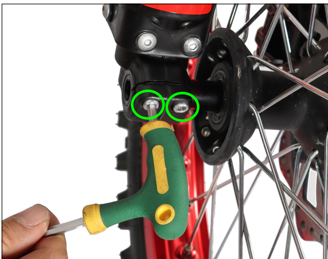
21. Tighten the two screws as shown in the picture to complete the tire locking process
