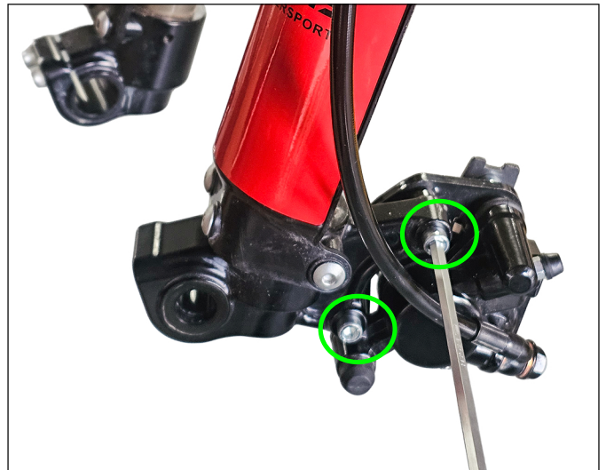
14. Unscrew the screws at two positions as shown in the figure to install and fix the brake
