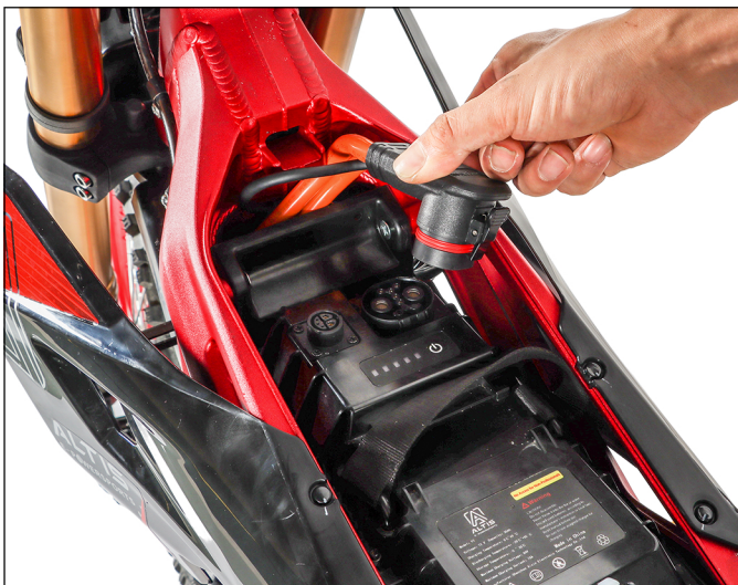
25. Insert the power cord into the battery socket
