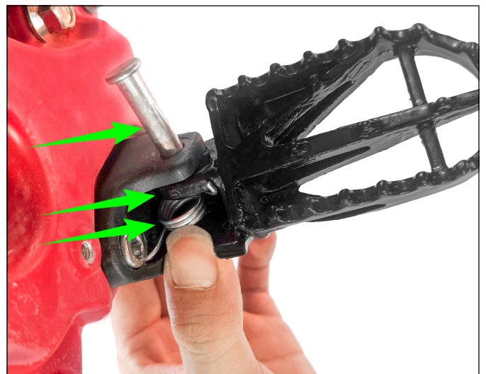
22. Loosen the screws and install the foot pedal As shown in the picture, the screw passes through the foot pedal and the spring
