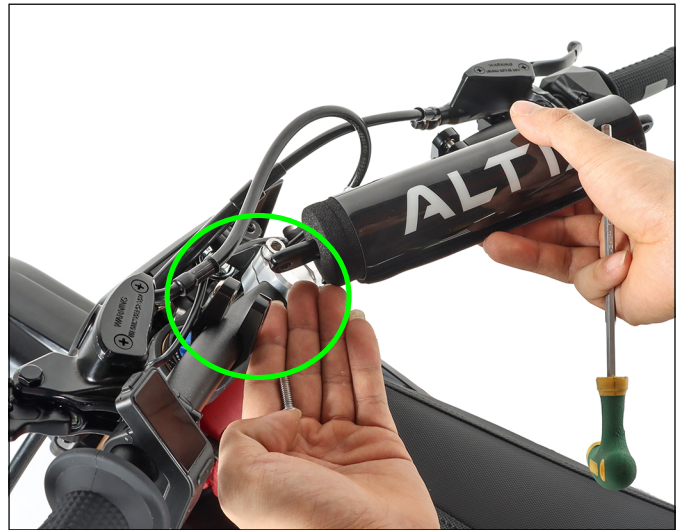
12. Remove the fixing screws to install the handlebar cushion pad
