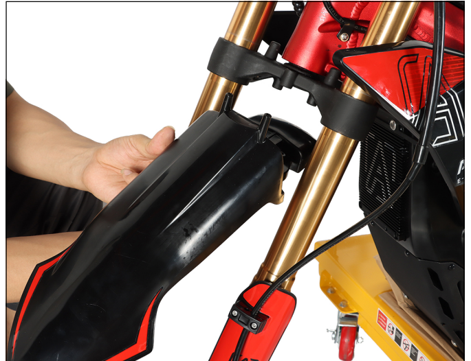
8. Remove the three screws from the mudguard hole and install the mudguard
