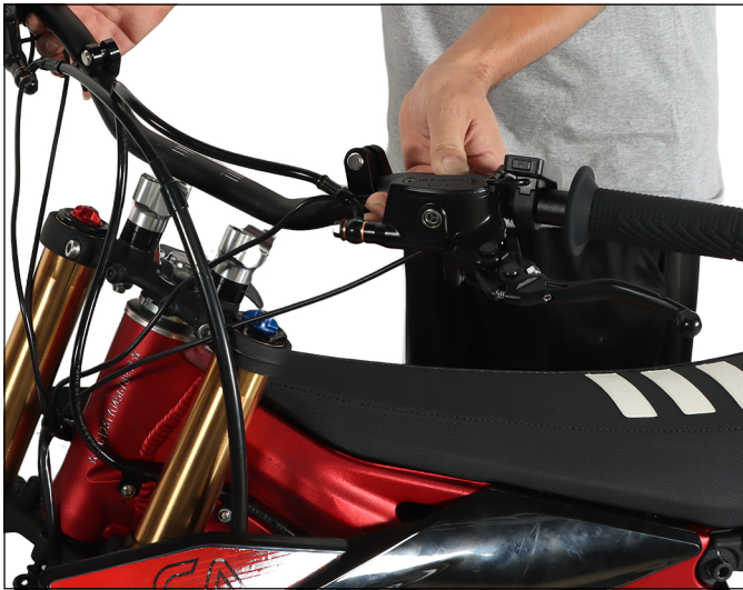
5. Remove the screws from the installation position of the handlebar and install the handlebar
