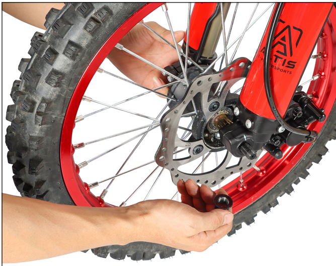
19. Insert the long rod and tighten the nut
