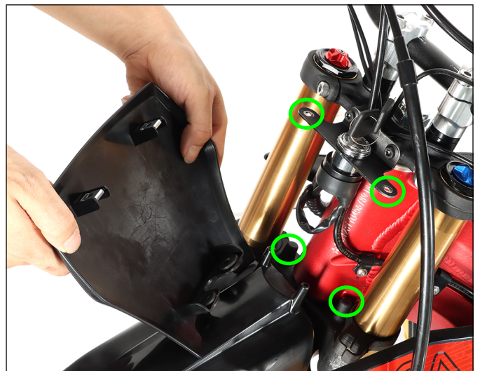
10. Install the corresponding bottom hole of the front face shield
