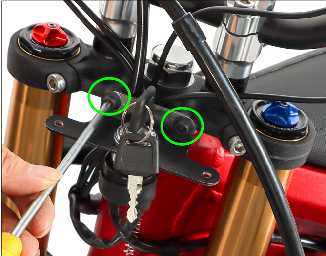
7. Unscrew the key switch screw to secure the position of the bracket key
