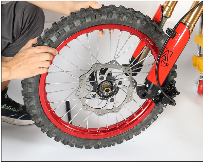
17. Observe the brake pad mount position and install the tire
