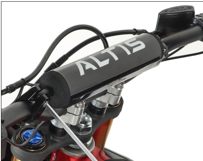
13. Unscrew the key switch screw to secure the position of the bracket key
