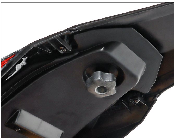
27. Lock the base screws tightly
