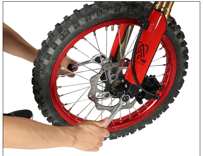
20. Fix and lock the tire on both sides simultaneously
